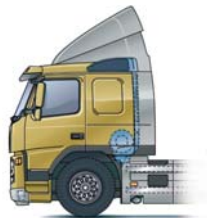
■ Sleeper cab with underrun protection, air intake, airflow package
