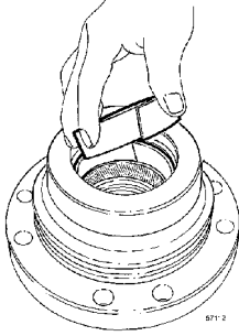
Figure 6 Installing bushes in piston rod guide
