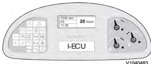
Figure 1 Instrument control unit with information display
