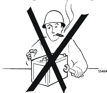
Figure 2 Do not smoke near batteries!
