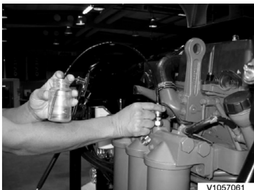
Figure 9 Example of sampling method with hose
