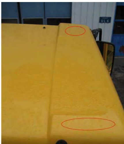
Fig. 1 Suggested antenna positions on roof.
