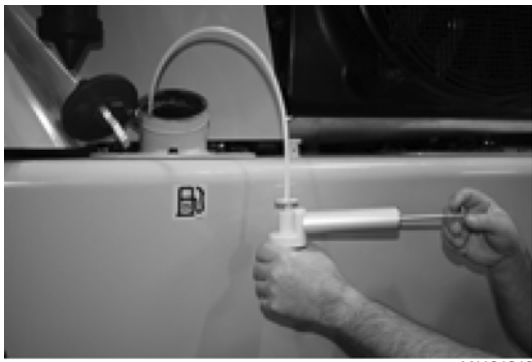
Figure 2 Example of fuel sampling
