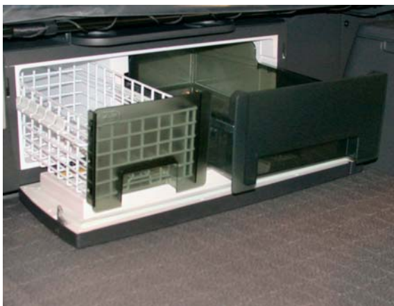
Refrigerator with freezer inside cab
