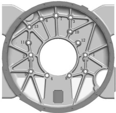
Fig. 4-11 Tightening Sequence of Flywheel Housing Bolt
