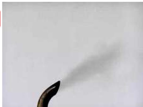
Fig.2-6 Check the exhaust gas
