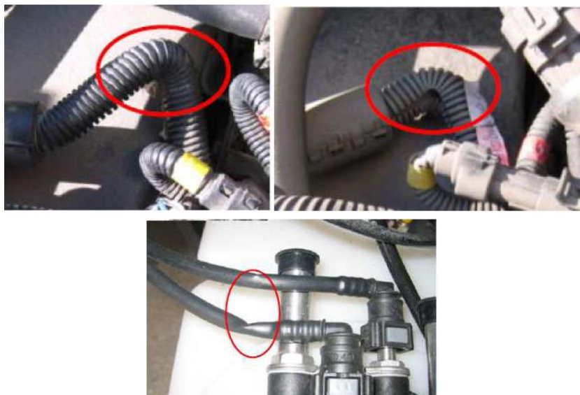
Fig. 4-76 AdBlue pipe severely bent
