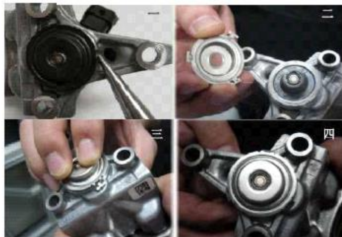
Fig. 4-70 Replacement of dosing module gasket
