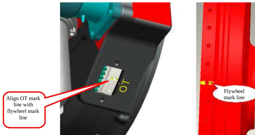
Fig.2-8 Flywheel mark line
