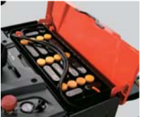
高性能的3PzS (4PzS) DIN标准电瓶, 适合长时间操作 The high-performance 3PzS (4PzS) DIN standard battery is suitable for long-time operations.
