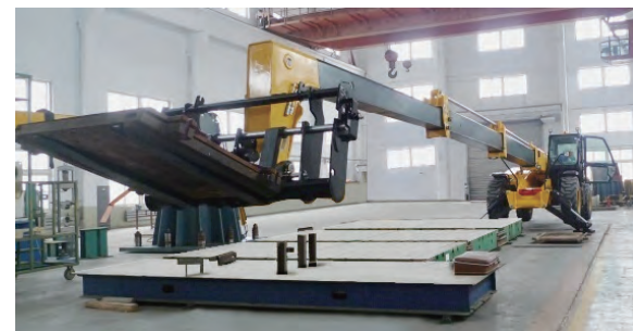
XC6-4517K 叉装机通过20万次疲劳载荷及超载试验 XC6-4517K has passed fatigue load and overload tests of 200,000 times
