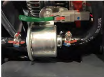
Fuel supply pump.
