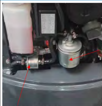
Fuel supply pump
