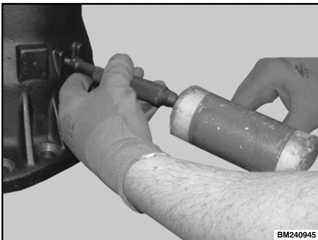
Figure 10. Installing the Breather
