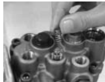
Install the spring, (delivery).
