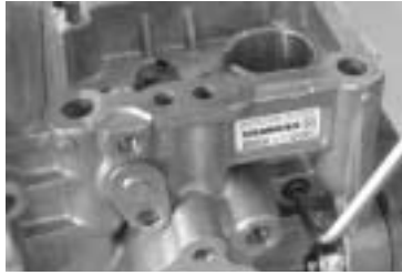
Remove the whirl-stop, (tappet).
