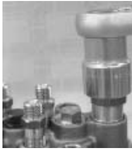
Fasten the thermo-element.
