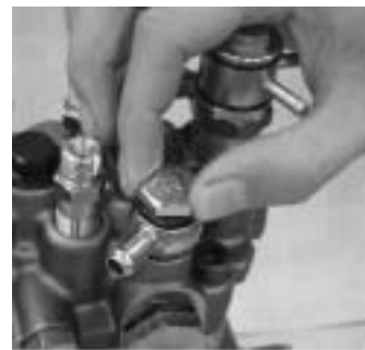
Install the joint, (FO inlet).
