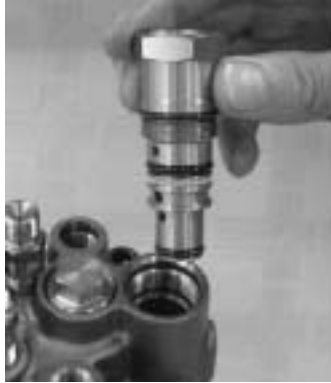
Install the holder with new O-ring, (timer).
