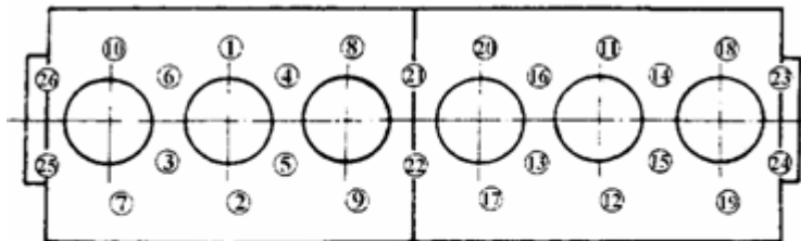
图 2-2 缸盖螺栓拧紧顺序 Fig 2-2 cylinder cover bolt tightening order
