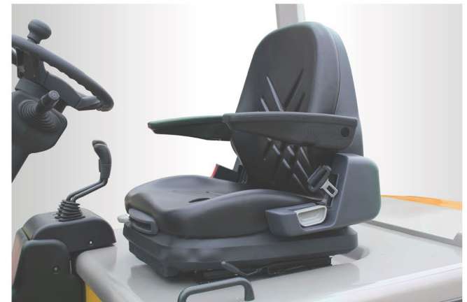
Optional sensing system on the seat to lock the working device when the operator leave the seat, which can avoid misoperation.
