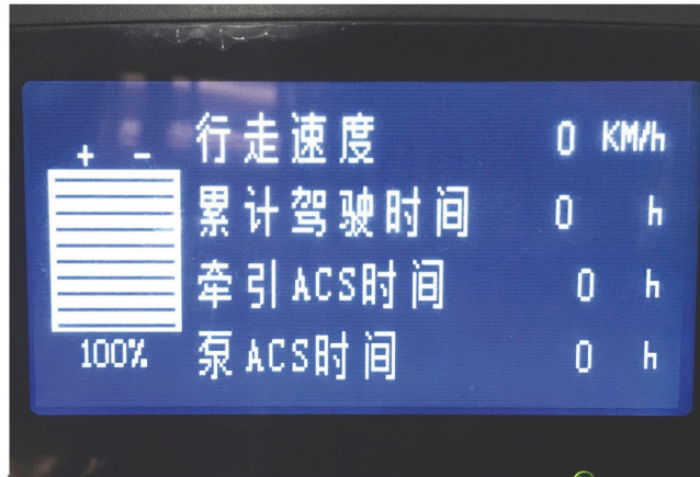
Curtis LED screen with settings of walking and lifting performance; it can monitor the running of motor, thus get working hours and fault code;
