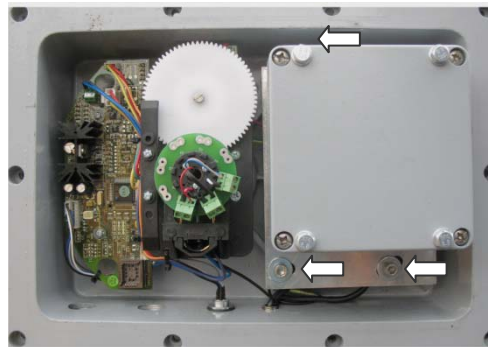
Angle sensor adjustment (see arrows above)
