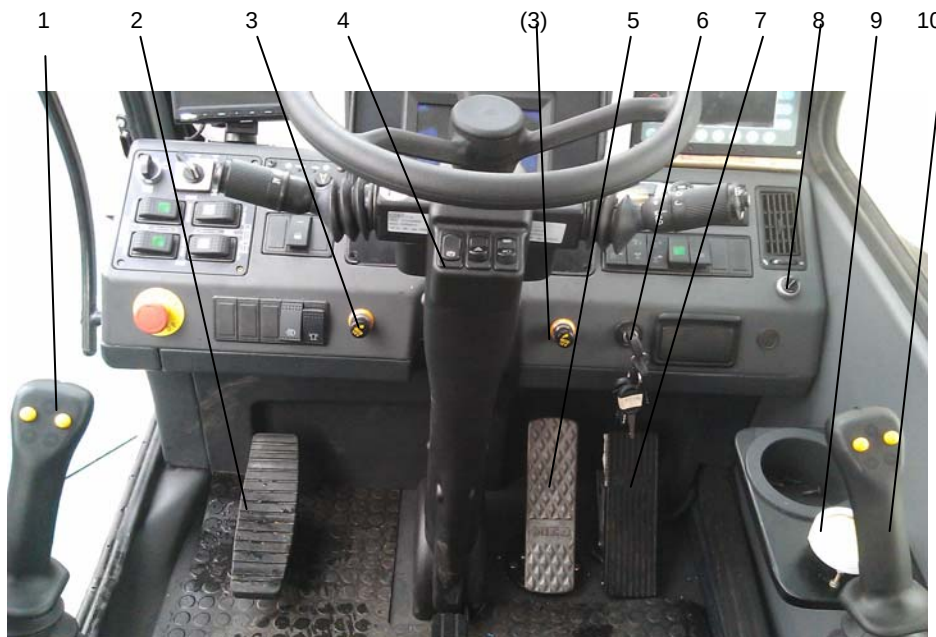
Figure 06 – 6 Controls and Instruments
