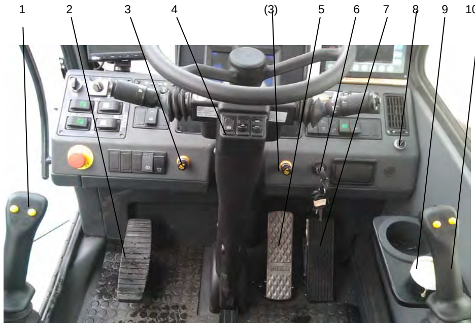
Figure 06 – 6 Controls and Instruments
