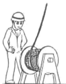
Figure 1-32 Monitor the Rope (Must Lay Flat and Evenly)
